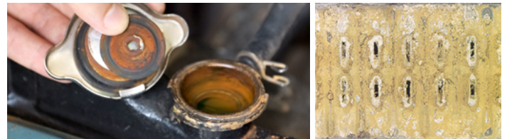
Corrosion in the cooling system
