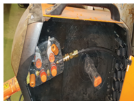
Connect the liner into the feeder adapter
