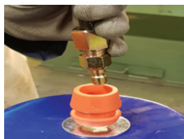
Click the liner onto the hood
