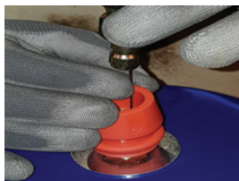
Feed the wire through the liner
